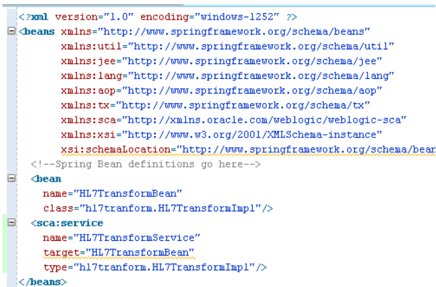
Illustration 56: Spring component configuration
