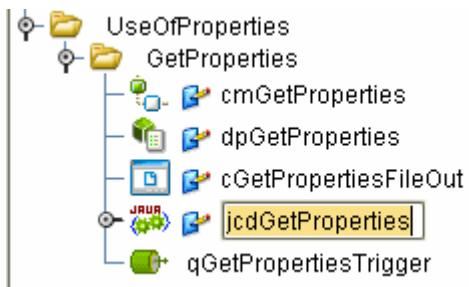
The JCD will be triggered by arrival of a message to a JMS Queue and will write output to a file using the File eWay.
