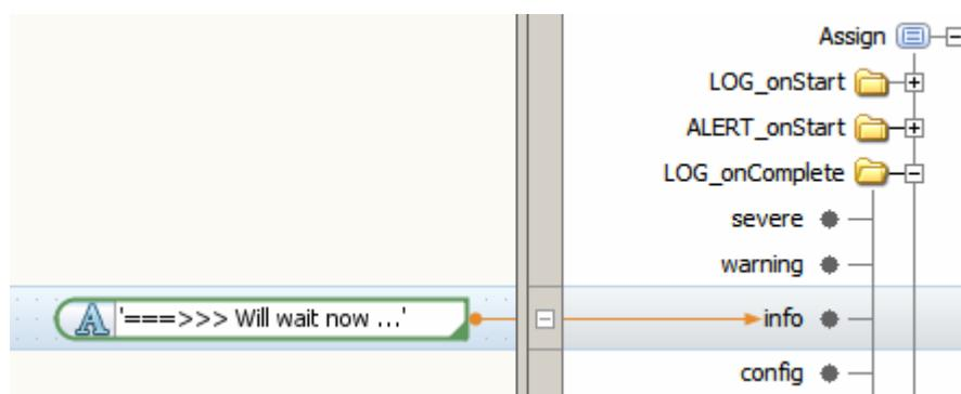
Switch to Design mode, select the Reply1 activity, switch to Logging mode and add logging text as shown:
